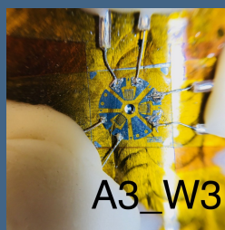
A3_W3 Strain gauge in place
