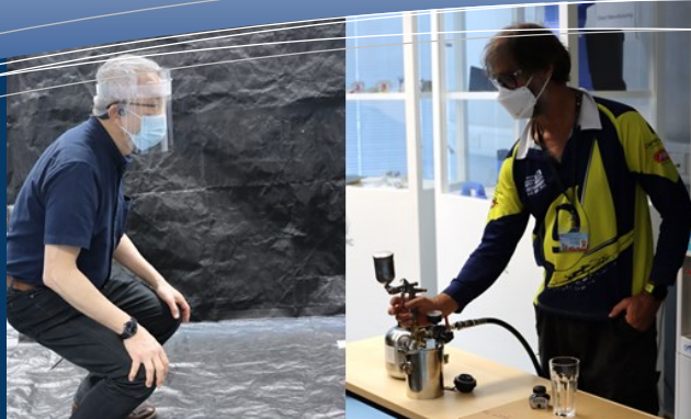
Testing Face shields with an artificial sneeze
